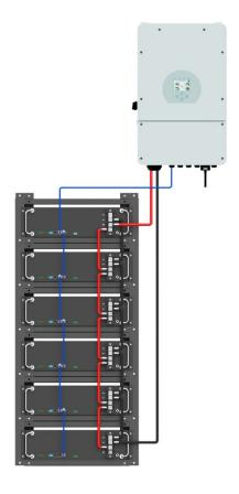
Figure 12. 6 batteries electrical installation diagram
