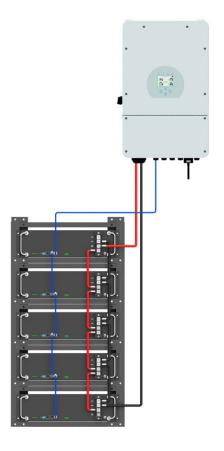
Figure 11. 5 batteries electrical installation diagram
