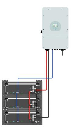
Figure 9. 3 batteries electrical installation diagram
