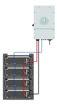
Figure 10. 4 batteries electrical installation diagram
