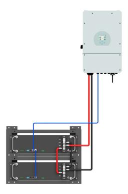
Figure 8. 2 batteries electrical installation diagram
