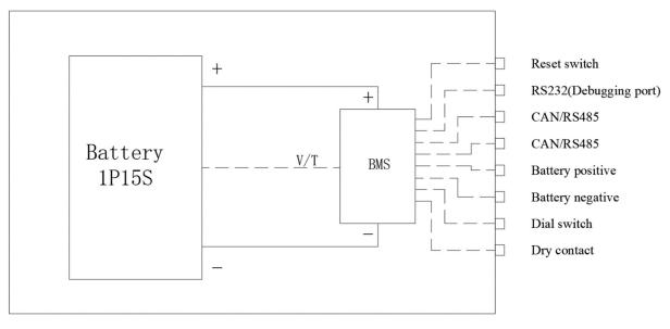
Figure 5. electrical schematic diagram of the product
