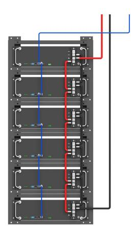
Figure 6. horizontal stacking installation diagram
